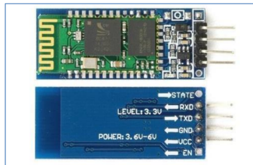
Figure 4. Bluetooth HC-06 Module
